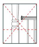
42" Rail Height = cut up to 8" off bottom of Post 36" Rail Height = cut up to 14" off bottom of Post
